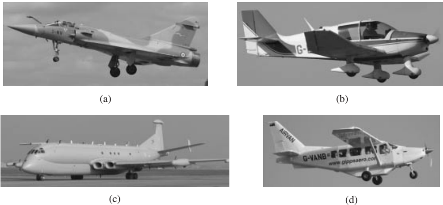
Figure 9.12 Four aircraft with various types of landing gear: (a) Dassault Mirage 2000 with retractable landing gear; (b) Robin DR-400-120 Dauphin with faired fixed landing gear; (c) Hawker Siddeley Nimrod with retractable landing gear; (d) Gippsland GA-8 Airvan with unfaired fixed landing gear. Reproduced from permission of (a, b, d) Jenny Coffey; (c) Antony Osborne
