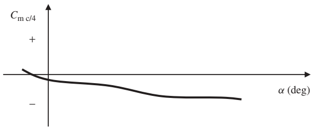
Figure 5.13 The variations of pitching moment coefficient versus angle of attack
