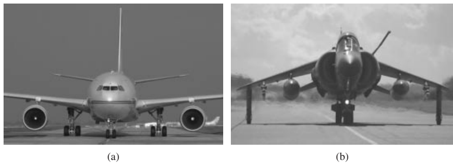
Figure 5.51 Two aircraft with different dihedral angles: (a) Airbus A330, dihedral; (b) British Aerospace Sea Harrier, anhedral (Reproduced from permission of (a) A J Best, (b) Jenny Coffey.)
